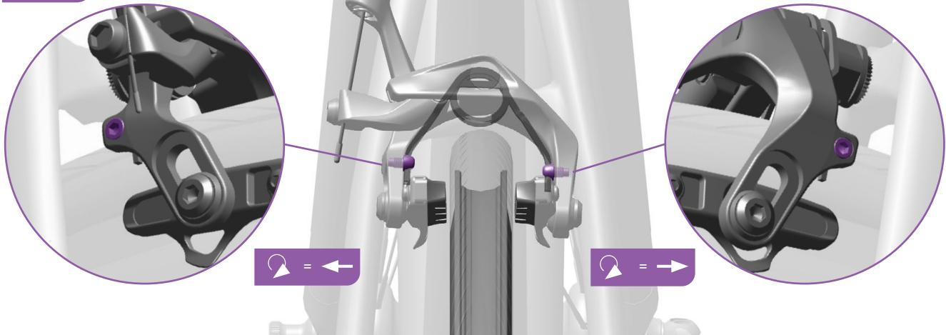
Center the brake pads on each side of the rim by adjusting the spring tension bolts.
