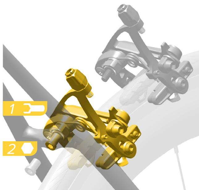
Install the caliper onto the frame or fork. Center the caliper on the rim and tighten the mounting nut enough that the caliper position can be easily adjusted.
