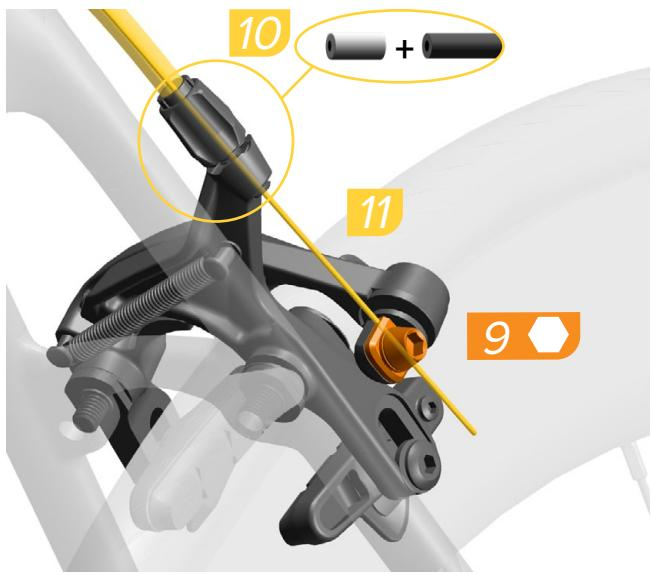
Install a 5 mm ferrule onto the housing, and install the cable and housing into the caliper barrel adjuster. Thread the cable into the groove of the cable clamp washer.
