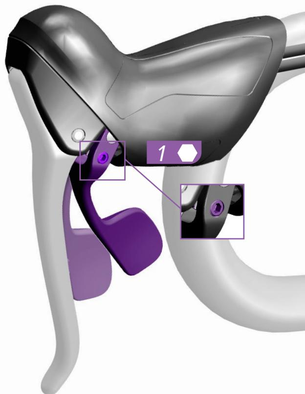
Adjust the Brake lever to the desired position. Leave a small gap between the shift lever and the brake lever.
