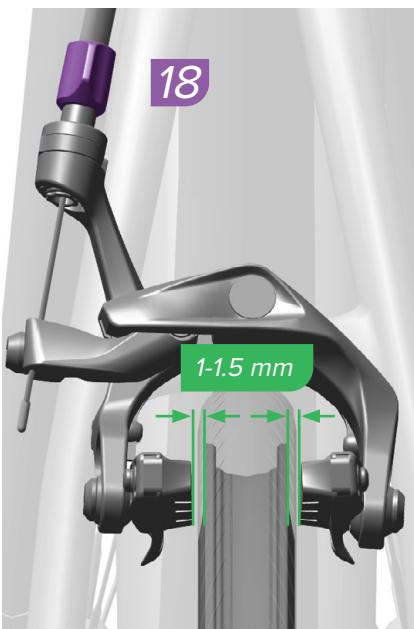
Turn the barrel adjuster until you have achieved the desired pad spacing and lever feel.
