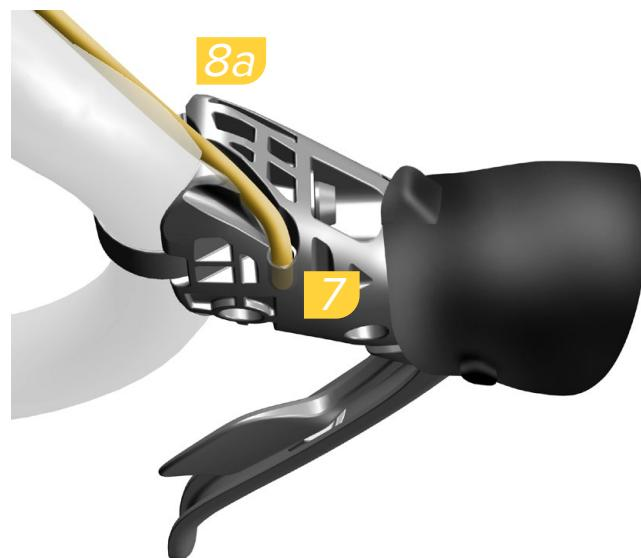
Install the shifter housing into the 4 mm factory installed ferrule. Route the housing in front of (8a) or behind the handlebar (8b) using the routing channels in the shifter.
