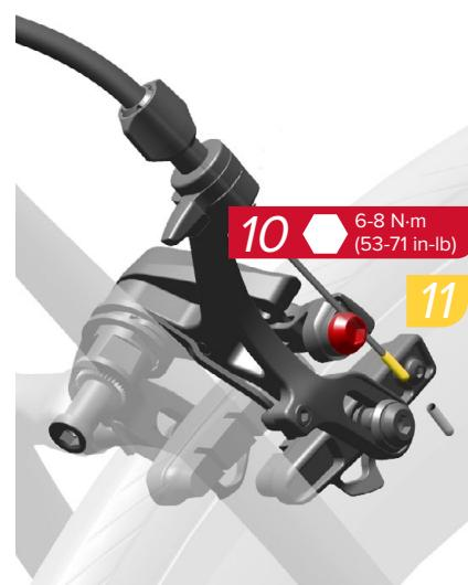
Install a 5 mm ferrule onto the housing, and install the cable and housing into the caliper barrel adjuster. Thread the cable into the groove of the cable clamp washer.
