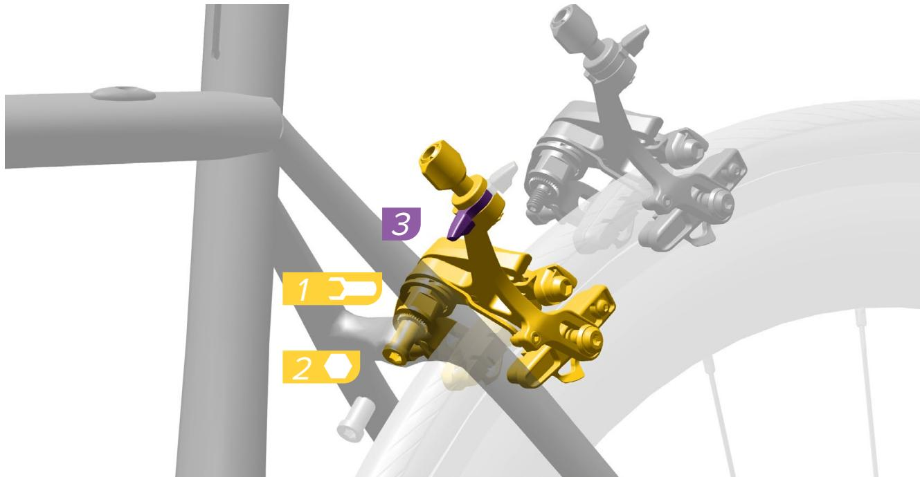
Install the caliper onto the frame or fork.
