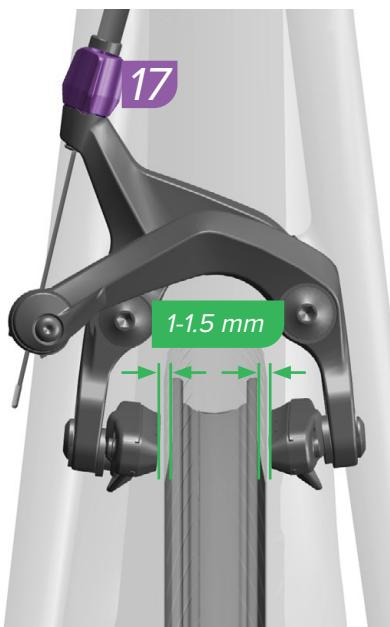
Turn the barrel adjuster until you have achieved the desired pad spacing and lever feel.
