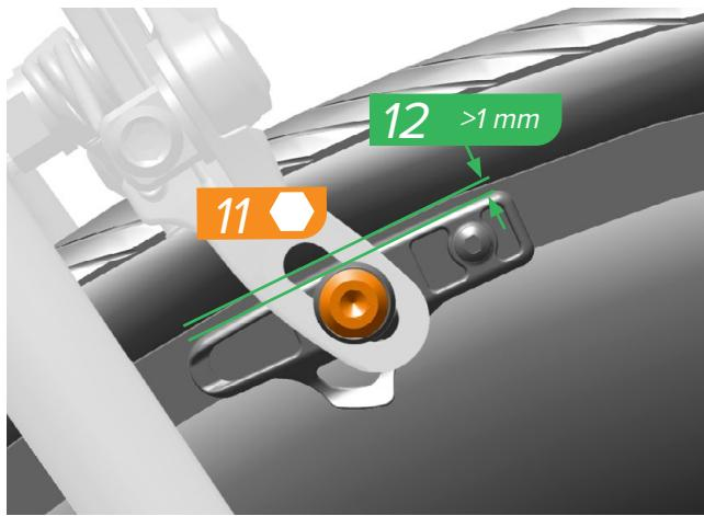
Loosen the brake pad bolt and position the brake pad so there is at least one millimeter between the brake pad and the top edge of the rim.
