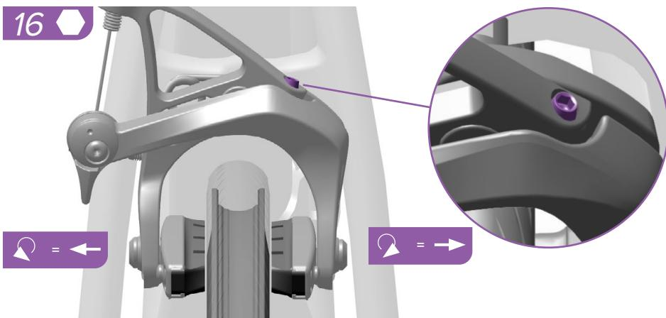
Adjust the spring tension bolt to center the brake pads on each side of the rim.
