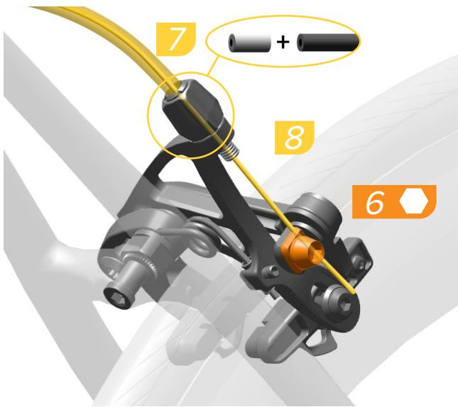
Install a 5 mm ferrule onto the housing, and install the cable and housing into the caliper barrel adjuster. Thread the cable into the groove of the cable clamp washer.
