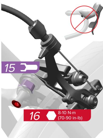
Hold the caliper centered on the rim, and tighten the mounting nut.
