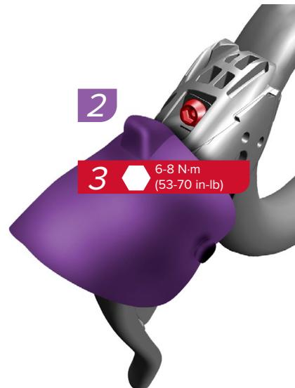
Fold the hood cover forward, then use a 5 mm hex to tighten the shifter bolt to 6-8 N·m (53-70 in-lbs).
