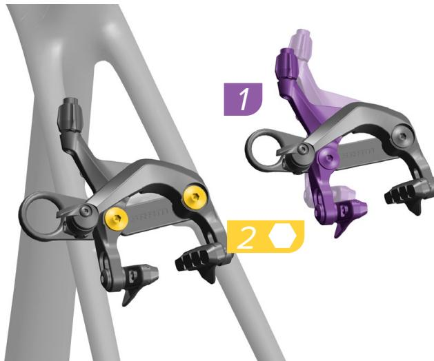
Squeeze the brake pads together to expose the left mounting bolt, then install the caliper onto the frame and thread each bolt in two full rotations.
