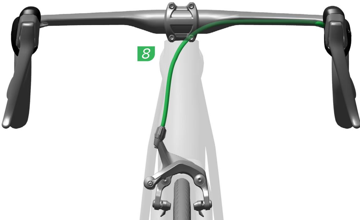
To determine where to cut the housing, hold the housing up to the shift-brake lever with a length that creates a gentle bend in the housing and allows the handlebar to freely turn from side to side.
