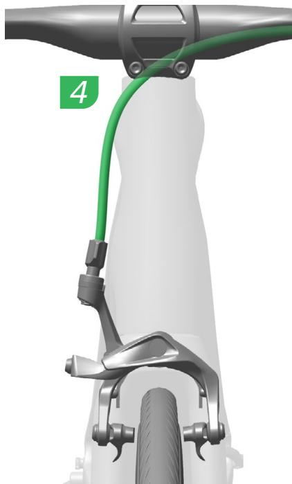
Make sure the housing is cut to the right length. If the housing length is too long, it will push the caliper away from a centered position. If the housing is too short, it will pull the caliper away from a centered position.
