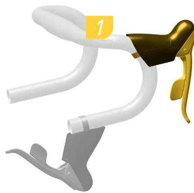
Install the shifter assembly onto the handlebar and set it to your desired position.
