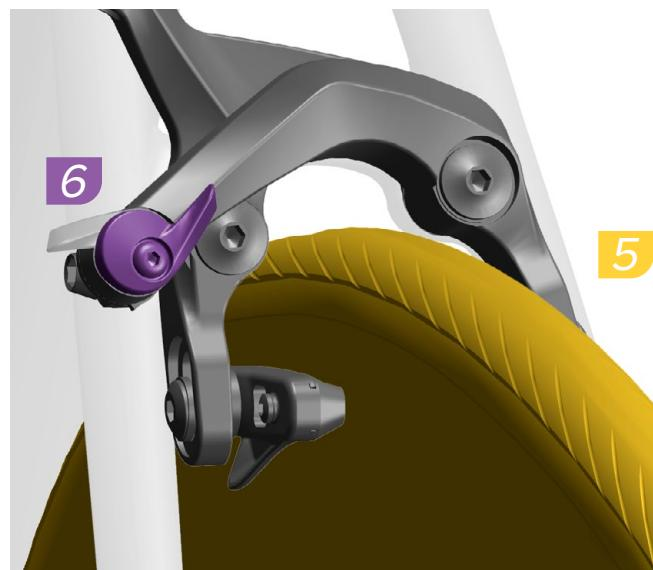
Adjust the centering bolt to achieve equal pad clearance on each side of the rim.
