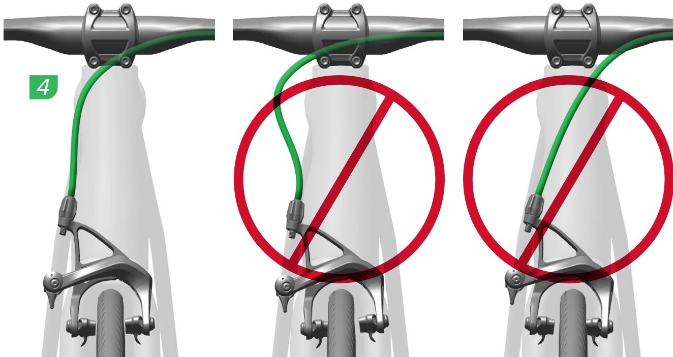
Make sure the housing is cut to the right length. If the housing length is too long, it will push the caliper away from a centered position. If the housing is too short, it will pull the caliper away from a centered position.
