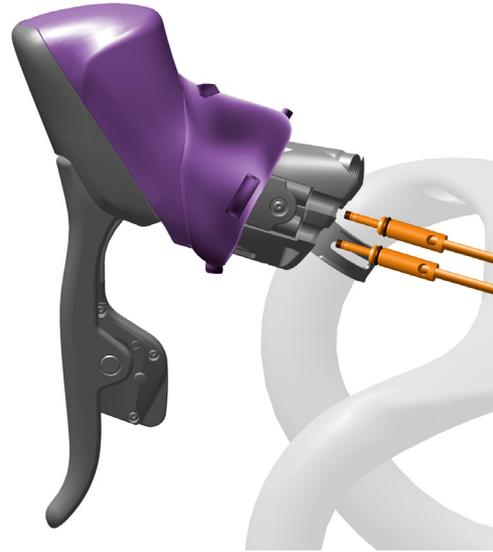
Remove the MultiClic wire connector from the AXS port. For MultiClics used with VukaShift AXS extension bars, consult the *VukaShift AXS User Manual* on [sram.com](http://sram.com).
