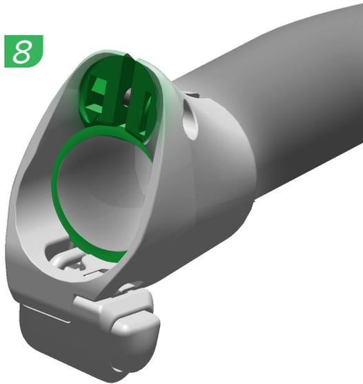
Install the ClampGrip on the handlebar so the edge of the handlebar is flush with the flat part in the ClampGrip. Tighten the ClampGrip.
