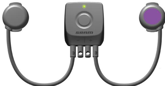
Press the right **+** Blip or Clic to move the rear derailleur outboard to a smaller cog. Press and hold for multiple shifts.
