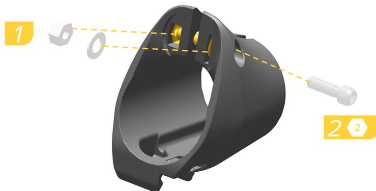
Install the washer and nut into the slots. Loosely install the bolt.
