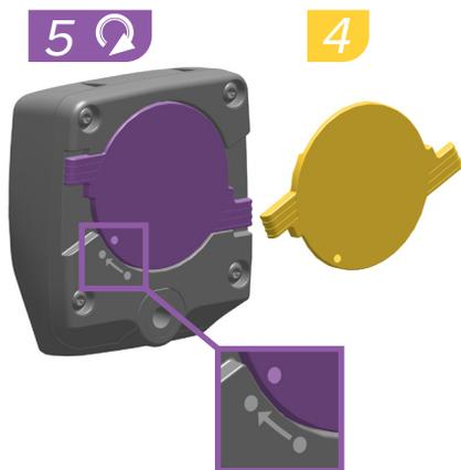
Reinstall the battery cap. Rotate the cap clockwise to align the dots and lock it into place.
