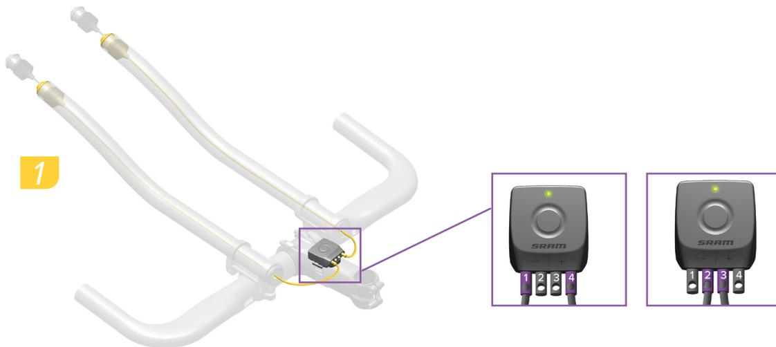
Install each Clic wire internally through the bar extension to the BlipBox.
