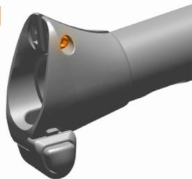
**For MultiClics with ClampClics:** Remove the brake according to the brake manufacturer's instructions. Use a 2 mm hex wrench to loosen the clamp bolt and remove the ClampClic.
