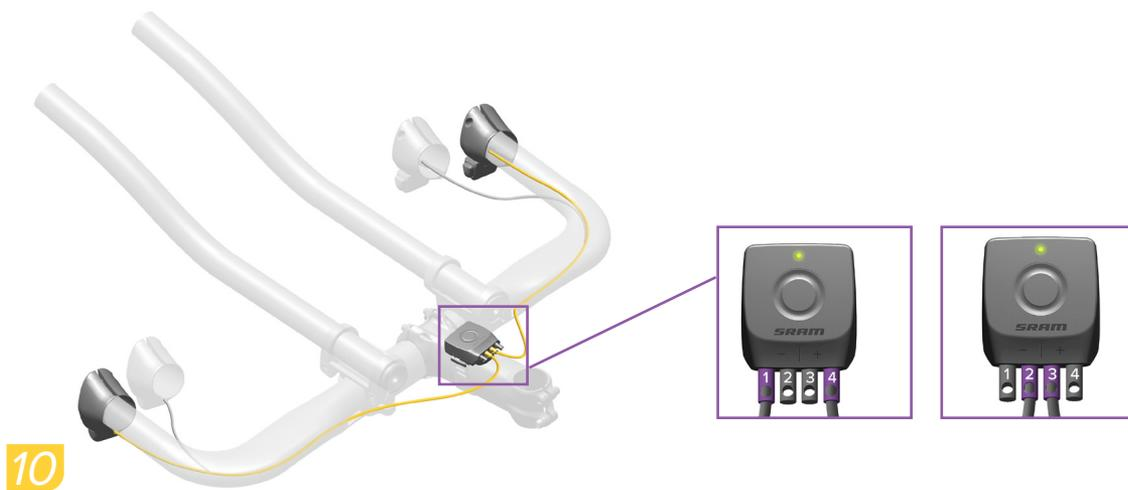
Route each MultiClic wire internally or externally to the BlipBox.
