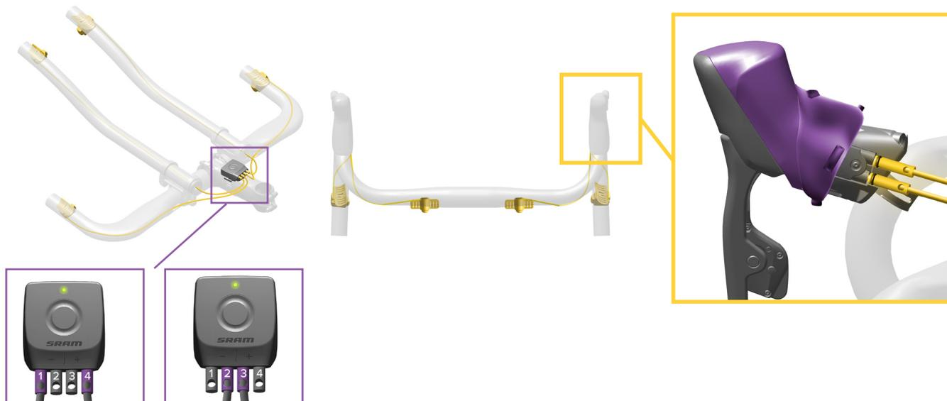
Route each MultiClic wire internally or externally to the BlipBox or AXS shifter. Insert each wire connector into the AXS shifter or BlipBox port 1 and 4, or 2 and 3. The wire connector is fully inserted when the detent is felt.
