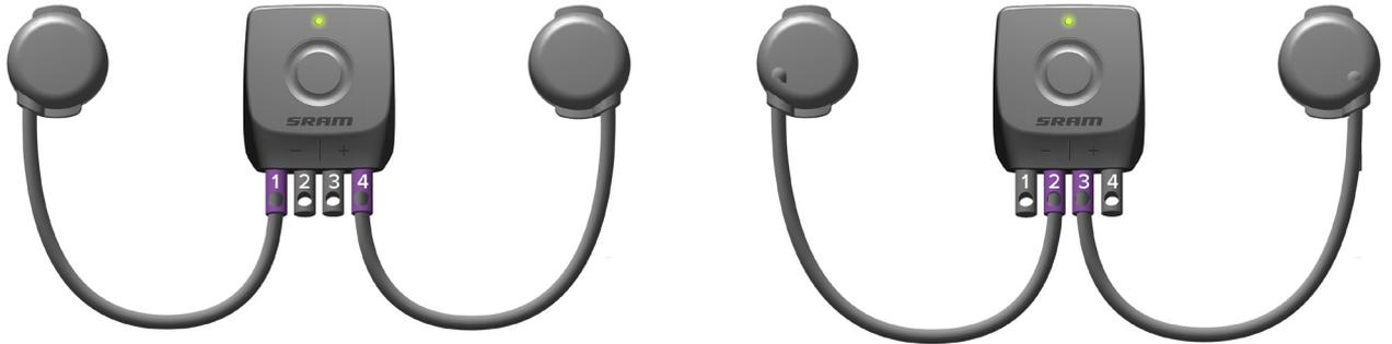
A remote shift button pair must be plugged into BlipBox AUX ports 1 and 4, or 2 and 3 to have Multipress functionality, a function when two remote shift buttons are pressed simultaneously.
