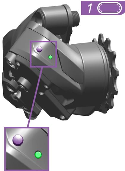
Begin the pairing session at the rear derailleur. Press and hold the AXS button on the rear derailleur until the green LED blinks slowly, then release.
