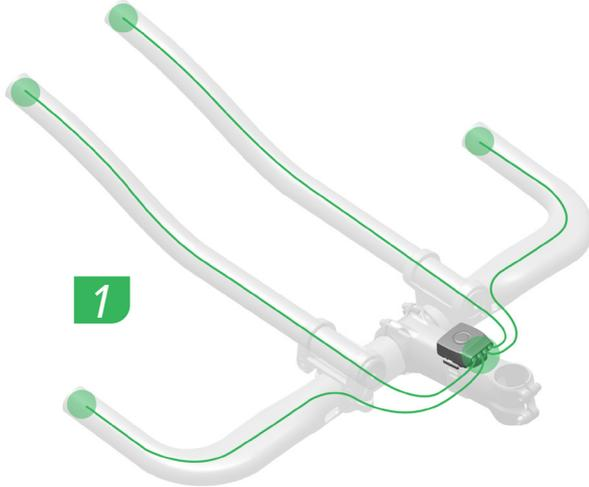
Measure the distance from the Blip location to the BlipBox and select the most appropriate Blip wire length from the available Blips.
