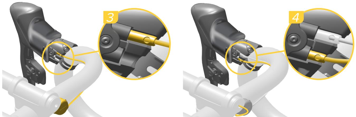
Route the wire from each Blip or Clic to the AXS shifter and insert the wire connectors into the AXS shifter. The wire connector is fully inserted when the detent is felt.
