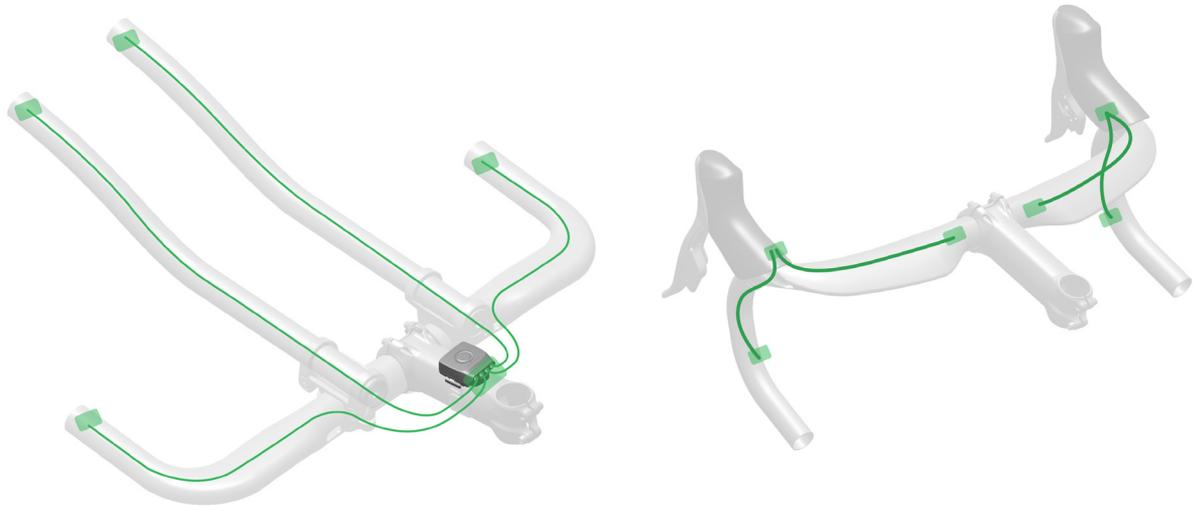
Measure the distance from the MultiClic location to the BlipBox and select the most appropriate MultiClic wire length.
