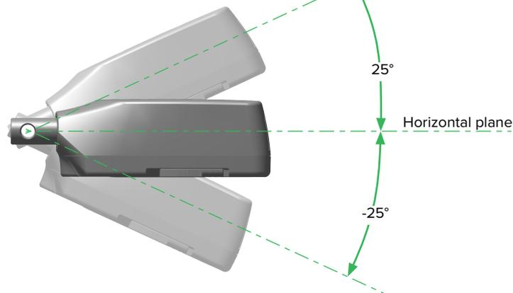
For optimal performance in an enclosed space, the BlipBox must be mounted within 25° of horizontal. The AXS button can face either up or down, and the wire inputs can face forward or backward.
