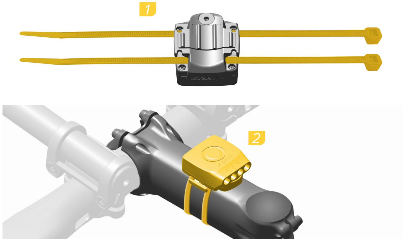
Insert plastic cable ties through the slots between the mount and the BlipBox, then attach the BlipBox to the bicycle. The BlipBox should be snug against the stem when the cable ties are installed.
