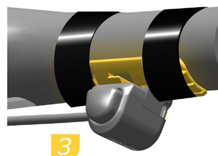
Use electrical tape to secure each MultiClic with wing to the handlebar, in the desired location. Make sure the MultiClic does not move when shifting.
