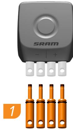
Remove one left **⊖** and one right **⊕** seal plug for each pair of Blips, Clics, or MultiClics to be installed.
