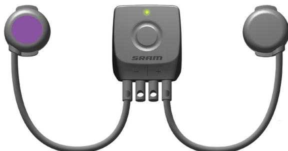
Press the left **-** Blip or Clic to move the rear derailleur inboard to a larger cog. Press and hold for multiple shifts.
