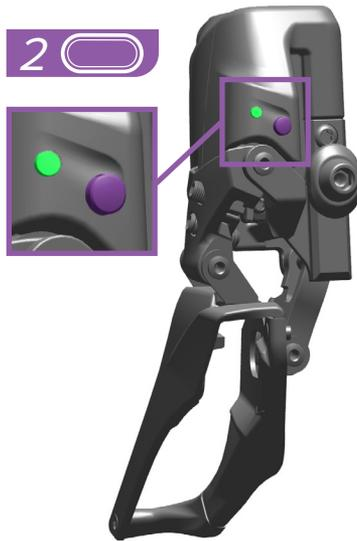
**For 2x systems:** Press and hold the AXS button on the front derailleur until the green LED blinks quickly, then release.
