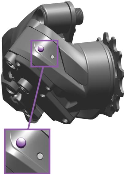
Press and release the AXS button on the rear derailleur to end the pairing session, or wait 30 seconds for the session to time out. The green LED will stop blinking.
