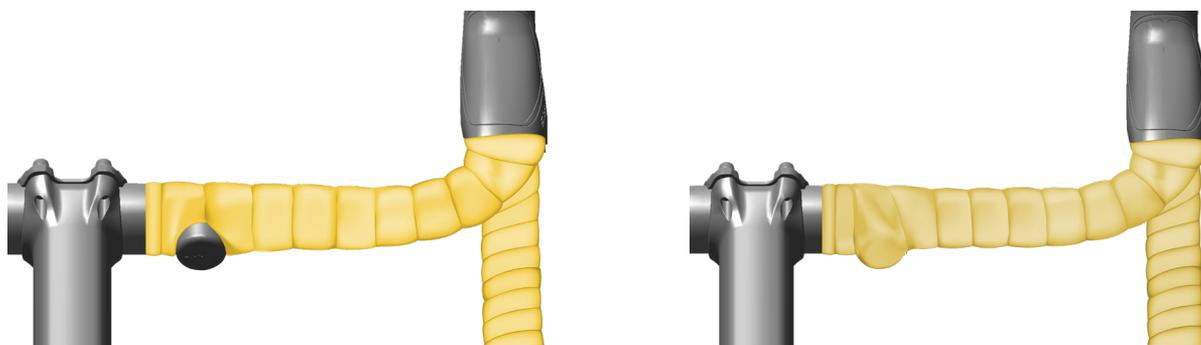
Wrap handlebar tape around or over the Blip to secure it to the handlebar or extension.
