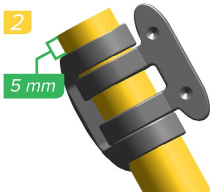
Apply Zipp Carbon Assembly Paste to the clamp contact surfaces.
