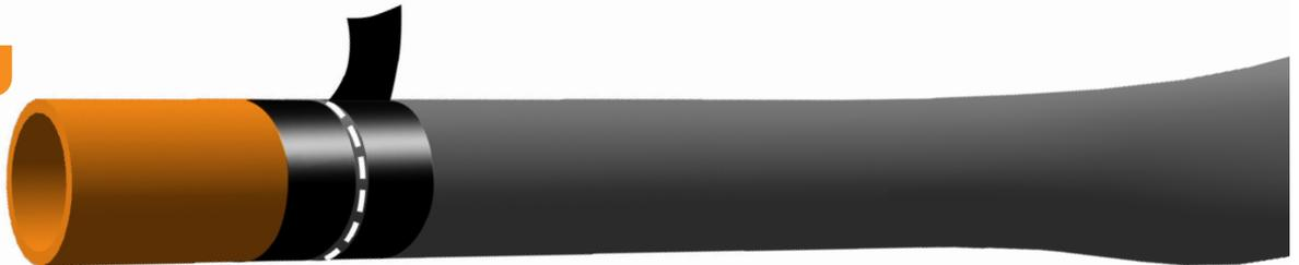
Wrap electrical tape around the extension on either side of the cut down line, leaving only a small gap between each piece of tape.
