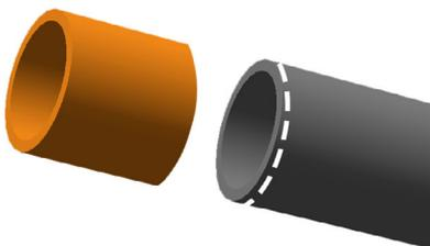
Use a saw guide and hacksaw to cut the extension to the desired length.
