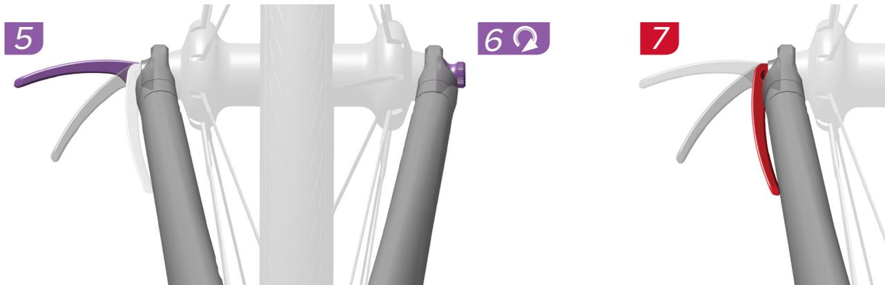
To increase lever tension, open the lever and turn the adjusting nut clockwise by hand. Close the lever to re-check lever tension. Lever tension is sufficient when the lever cannot be rotated while in the closed position. If the lever can be rotated while in the closed position, this is an indication that lever tension is insufficient and must be increased.
