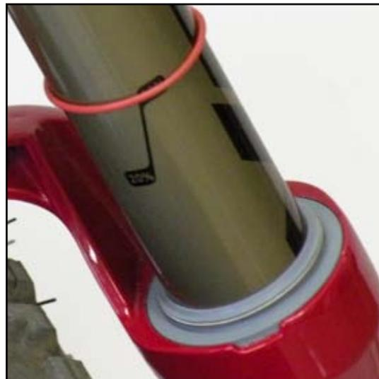
If you are unable to tune your fork to sag within the indicated range, you may need to change the coil spring (coil spring tuning). Use the specific tuning information that follows to achieve proper sag.
