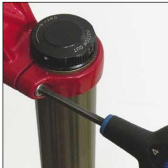
**2** Use a 1.5 mm hex to loosen the two set screws that retain the Bottom Out adjuster knob located on the top of the non-drive side fork leg (it is not necessary to remove the set screws). Remove the Bottom Out adjuster knob.
