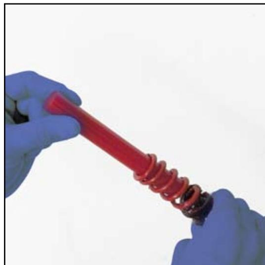
**7** Identify the tightly wound end of the new coil spring. Use a grease brush and apply a generous amount of grease to the entire length of the new coil spring. Install the coil spring, with the tightly wound end first, into the upper tube.
