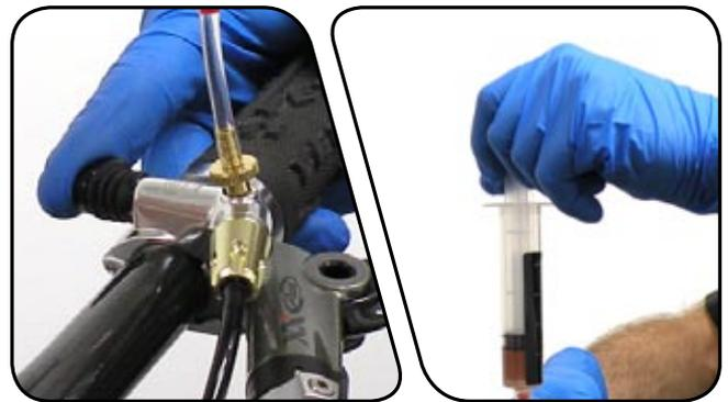
**15** Push in on the syringe plunger, and then press in the XLoc button to release it to the locked position. t
