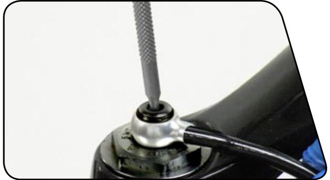
**13** Hold the XLoc button in the extended (locked) position and pull out the syringe plunger. Small bubbles will move into the suspension fluid as air is pulled from the system.
