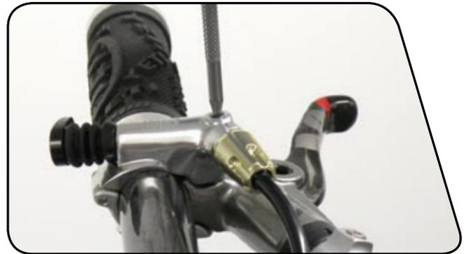
**10** Apply a few drops of suspension fluid to the XLoc bleed port, and then thread the brass fitting of the other speed lube kit into the bleed port.
