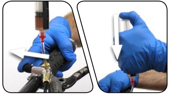
**16** Repeat steps 13-15 until air bubbles no longer move into the suspension fluid. It can take several repetitions of this process to fully void the system of air.
